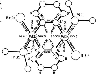
planes is 79°. Thus the approximate symmetry of the molecule is  $C_2$ . The long Pd...Pd distance of 3.194(2)  $\mathring{A}$  implies no bonding interaction between the metal atoms.
